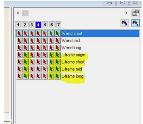
ii. To make a selection, select L-Frame Origin from the list, move the cursor over the large camera view where the L-Frame is visible, get as close to the origin marker as possible, **LEFT CLICK AND HOLD THE LEFT CLICK**, then utilize the lower right hand zoomed in camera view to get as accurate as possible with your selection, then release the left click to make your selection.
